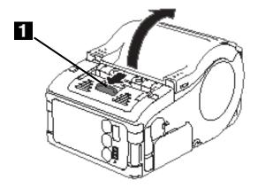
3. If the lever is not accessible, first slide the dispenser unit away by lifting the top edge where the arrow marks are located. (see Step 1 of "Loading the Label Roll" on page 30).
